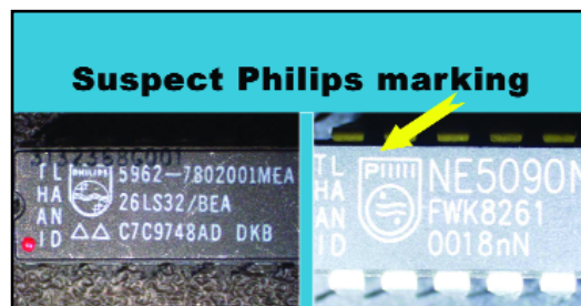
Suspect Philips marking covers old Philips marking for a different part.
